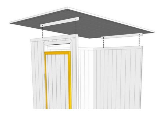
Drill through holes on the L-shaped profiles and on the wall for anchor the roof to the structure by means of steel bolts inox N.B.: the most protruding part of the roof with respect to the L profile,
