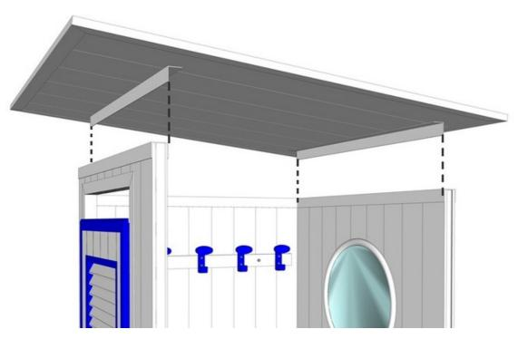
P.N.: the most protruding part of the roof with respect to the L profile, It must face the front.
